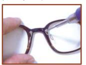
Put the CNPA pad arms back in the pin slots and using the self-tapping screws that come with the set, tighten the pad arms against the frame.
