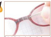
Detach the temples from the frame. Once you have cut off the formed nose pads, with cutters, filed down, and polished any remaining burrs, use the grid sheet to determine the insertion point of the Titarm.
